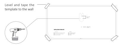
Drill three screw holes in the wall and remove the instruction tamplate
